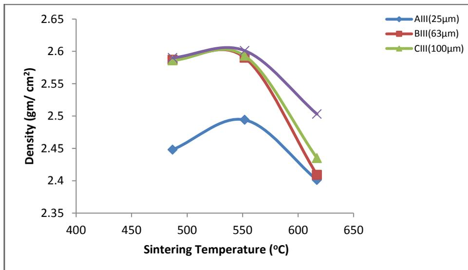
Figure. 4 the relationship between the sintering temperature and the density for different particle sizes.
