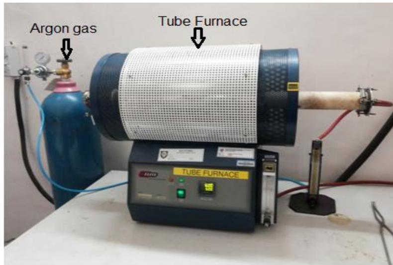
Figure. 2 Sintering furnace.
