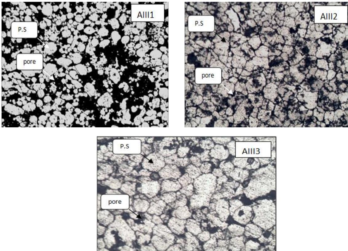
Figure. 7 effects sintering temperature on Microstructure of AIII (25 μm powder)
