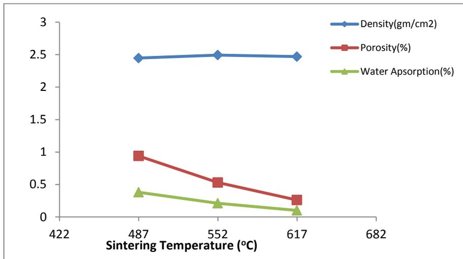
Figure. 3 relation between Sintering temperature and Physical properties
